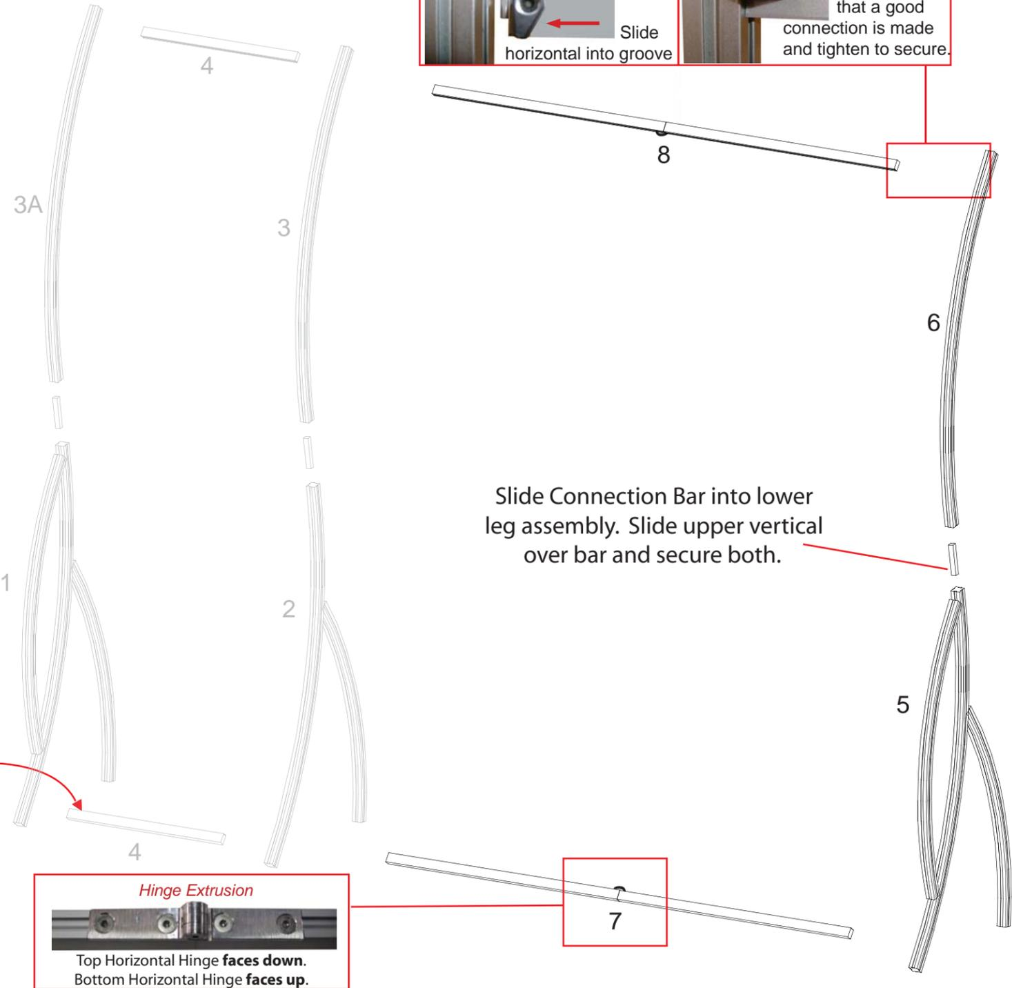
Slide Connection Bar into lower leg assembly. Slide upper vertical over bar and secure both.
